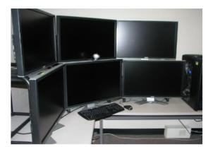
A high powered desktop system, DeepSix employs a tiled display of six 30 inch Dell monitors capable of a 2560×1600 resolution each. At a combined resolution of 7680×3200, this is our highest resolution single display available in the lab.
