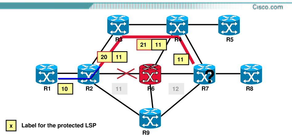
The Point of Local Repair learns the label to use from the Record Route Object object carried in the Resv message when the reroutable LSP is first established – Global Label Allocation must be used.
