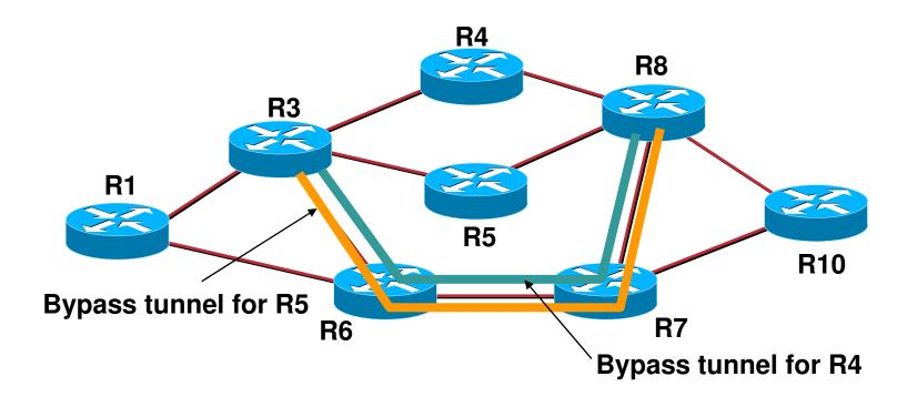
Only need to allocate enough BW on R3-R6-R7-R8 to protect for a single node failure – "N:1" protection
