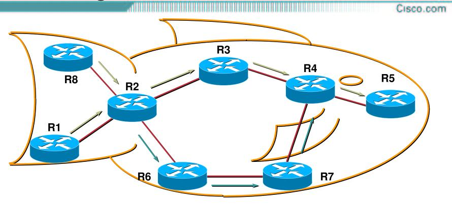
IP (Mostly) Uses Destination-Based Least-Cost Routing Flows from R8 and R1 Merge at R2 and Become Indistinguishable From R2, Traffic to R3, R4, R5 Use Upper Route
